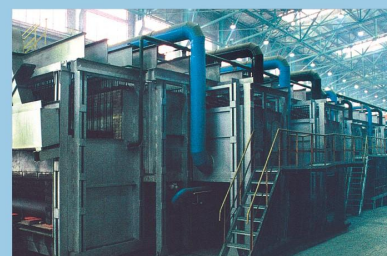
60m annealing furnace
