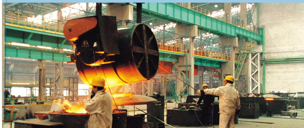
Heating and spheroidization in induction furnace
